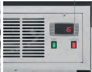
Electronic temperature controller
