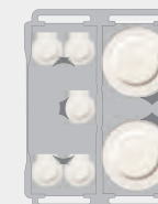
5 columns - plates of \varnothing 102 mm 2 columns - plates of \varnothing 334 mm 2 columns - plates of \varnothing 230 mm
